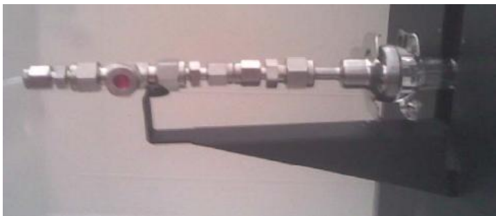
Figure 2 — Inserting a T with a septum in the carrier gas line of a Sunset Laboratory OCEC Lab instrument.
