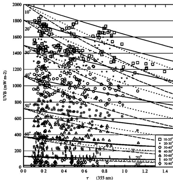
**Figure 10.** Measured Brewer and Bentham UVB dose rates versus aerosol optical depth at 355 nm for various solar zenith angle intervals. The various lines are model calculations for fixed solar zenith angles, an ozone column of 340 Dobson Units (DU) and Ångström coefficient  $\alpha = 1.0$ . The aerosol single-scattering albedo was 0.95 (solid line), 0.87 (dotted line), and 0.80 (dashed line).
