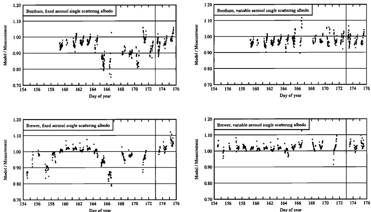
**Figure 5.** Model/measurement ratio for global irradiance integrated over UVA (315–365 nm) as a function of time. (left) Fixed aerosol single-scattering albedo,  $\omega = 0.87$ , used for the model simulations. (right) The aerosol single-scattering albedo was varied from day to day as shown in Figure 6. After day 171 (vertical line) both instruments were colocated in Tatoi, Athens. A total of 390 (454) Brewer (Bentham) measurements are compared with model simulations.
