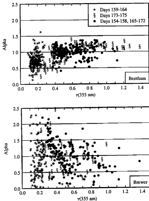
**Figure 2.** Ångström coefficient  $\alpha$  versus the aerosol optical depth at 355 nm,  $\tau(355 \text{ nm})$ , as measured by the (top) Brewer and (bottom) Bentham instrument. For days 173–175, both instruments were colocated in Tatoi, Athens.
